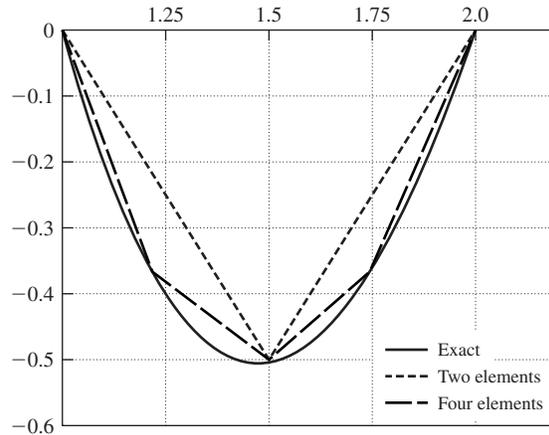
**Figure 5.6** Two-element, four-element, and exact solutions to Example 5.5.
