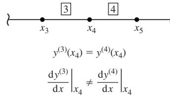
**Figure 5.5** Two elements joined at a node.
