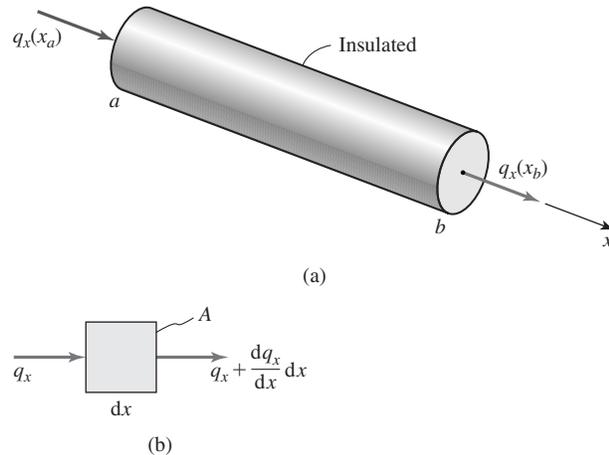
**Figure 5.8** Insulated body in one-dimensional heat conduction.
