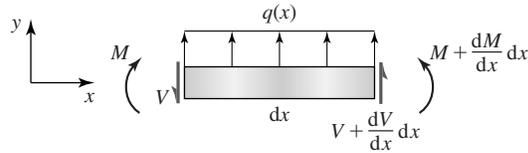
**Figure 5.7** Differential section of a loaded beam.
